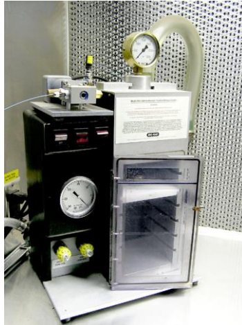
Figure 5. An example of a “gene gun” used for biolistics
